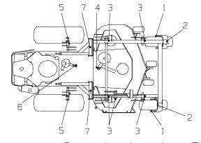
c) Lubricate front caster pivots once a year. Remove hex plug and cap. Thread grease zerk in hole and pump with grease until it oozes out around top bearing. Remove grease zerk and thread plug back in. Place cap back on.
